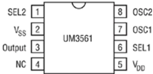
Figure 1.2 above shows the pin configuration of the IC UM3561
